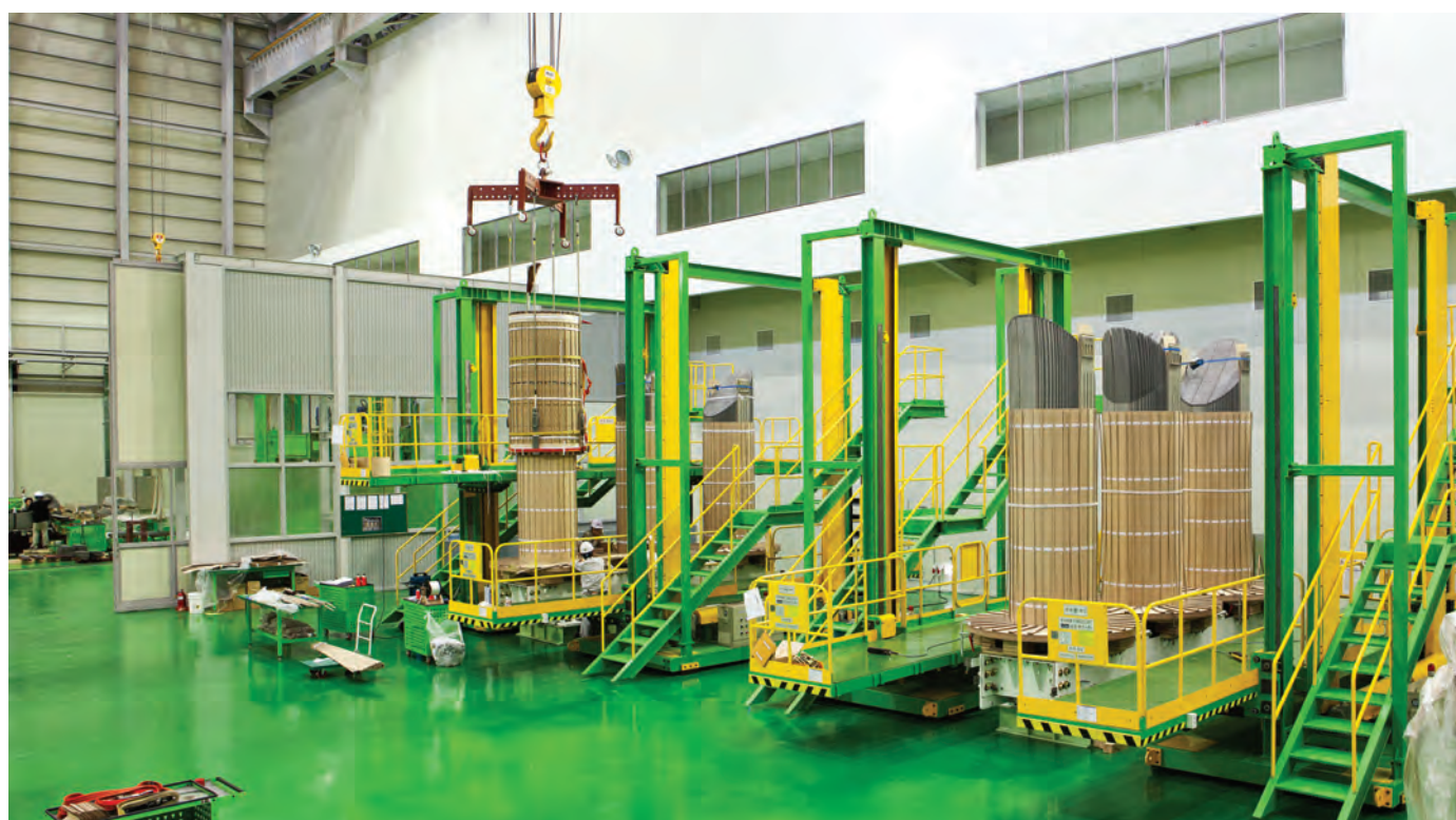
· CORE AND COIL ASSEMBLY SHOP
