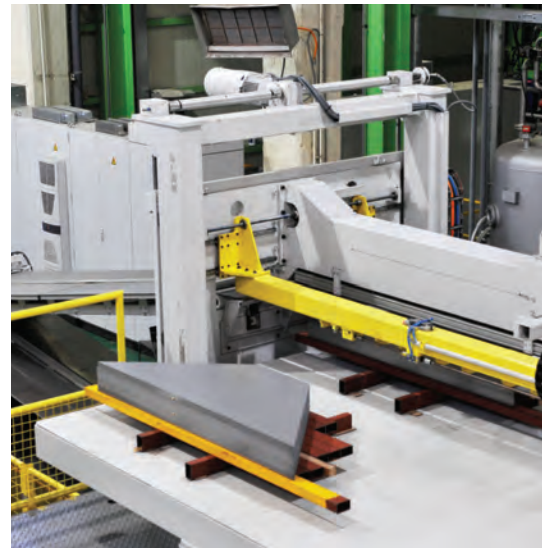
· AUTO CORE CUTTING MACHINE (CUT TO LENGTH)
