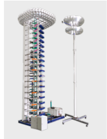
Impulse testing equipment up to 3600kV
